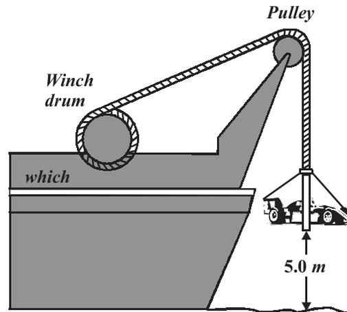
16. A  $2000 \text{ kg}$  block is lifted by a steel cable which passes over a pulley to a motor-driven winch (see fig 9.22). The radius of the winch drum is  $30 \text{ cm}$ , and the moment of inertia of the pulley is negligible.
