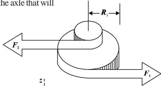
10. A wheel is rotating clockwise on a fixed axis perpendicular to the page. A torque that causes the wheel to slow down is best represented by the vector
