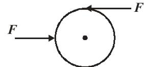
22. In the figure, the rotational inertia of the wheel and axle about the center is  $12.0 \text{ kg} \cdot \text{m}^2$ , the constant force  $F$  is  $39.2 \text{ N}$ , and the radius  $r$  is  $0.800 \text{ m}$ . The wheel starts from rest. When the force has acted through  $2.00 \text{ m}$ , the rotational velocity  $\omega$  acquired by the wheel due to this force will be
