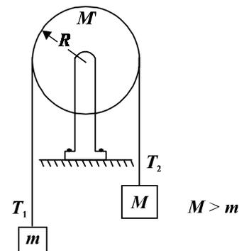
13. The moment of inertia of the wheel in the figure is  $0.50 \text{ kg} \cdot \text{m}^2$ , and the bearing is frictionless. The acceleration of the 15-kg mass is approximately
